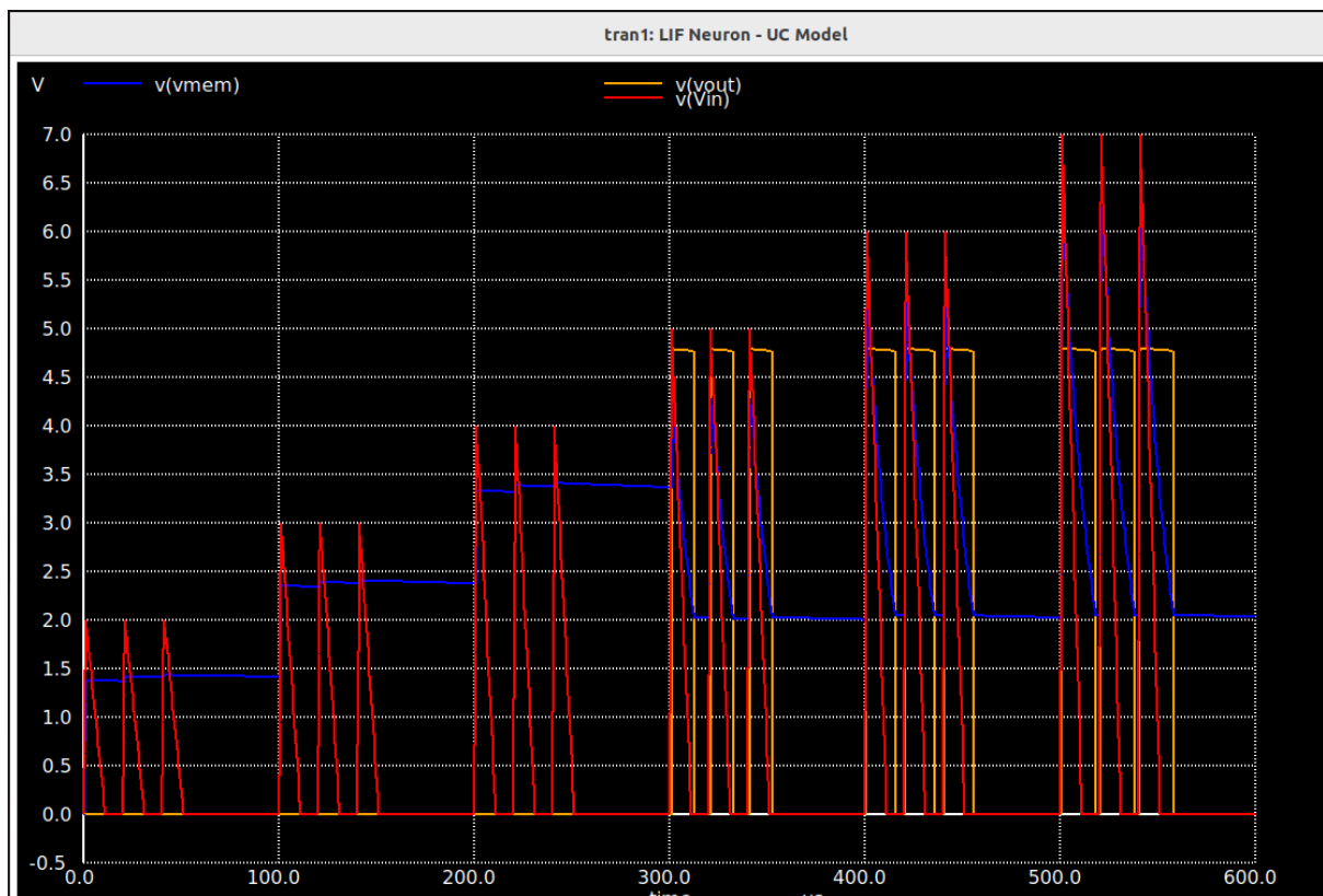
Fig. 6: Combined Waveforms ( V_{in} , V_{mem} , V_{out} )
