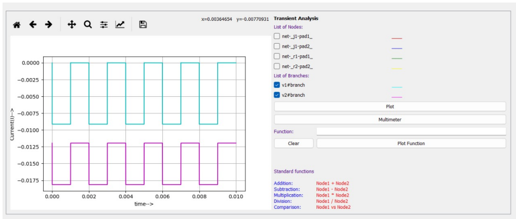
Figure 2: Ngspice transient simulation output showing gate and drain voltage waveforms.
