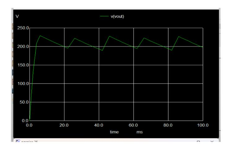
Fig 5 : The output waveform shown in Figure 5 illustrates the pulsating direct current (DC) produced by the bridge rectifier. This waveform exhibits reduced ripple due to the smoothing effect of the capacitive filter, resulting in a more stable DC output suitable for powering electronic devices.
