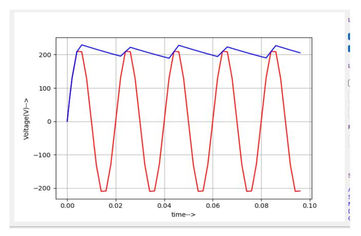
Fig 6: The output waveform shown in Figure 6 illustrates the pulsating direct current (DC) produced by the bridge rectifier. This waveform exhibits reduced ripple due to the smoothing effect of the capacitive filter, resulting in a more stable DC output suitable for powering electronic devices.
