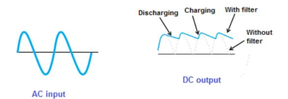
Fig 2: Input and Output of the Bridge Rectifier
