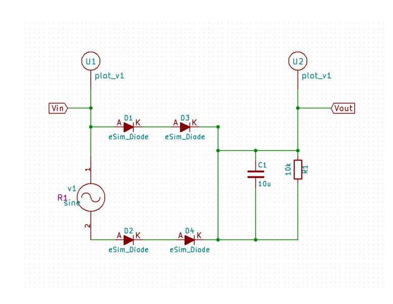
Fig 3: Shows a bridge rectifier circuit with four diodes that converts AC input into pulsating DC output. A capacitive filter is connected in parallel with the load to smooth the output voltage, reducing ripple and ensuring a stable DC supply.
