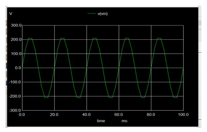
Fig 4: The input waveform depicted in Figure 4 represents the alternating current (AC) signal, characterized by its sinusoidal shape. This waveform is fed into the bridge rectifier, where it will be converted into a pulsating direct current (DC) output.
