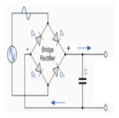
Fig 1: Bridge Rectifier
