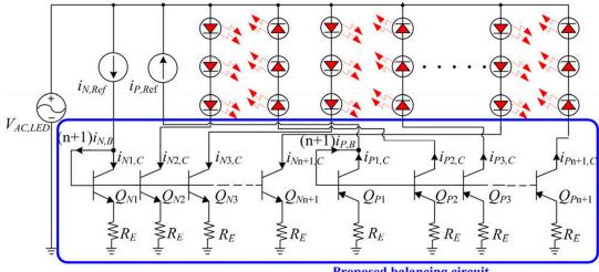
Proposed balancing circuit
