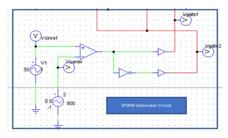
**Title of the paper:** Sine Wave Inverter Bipolar SPWM using Analog Triggering Circuit
