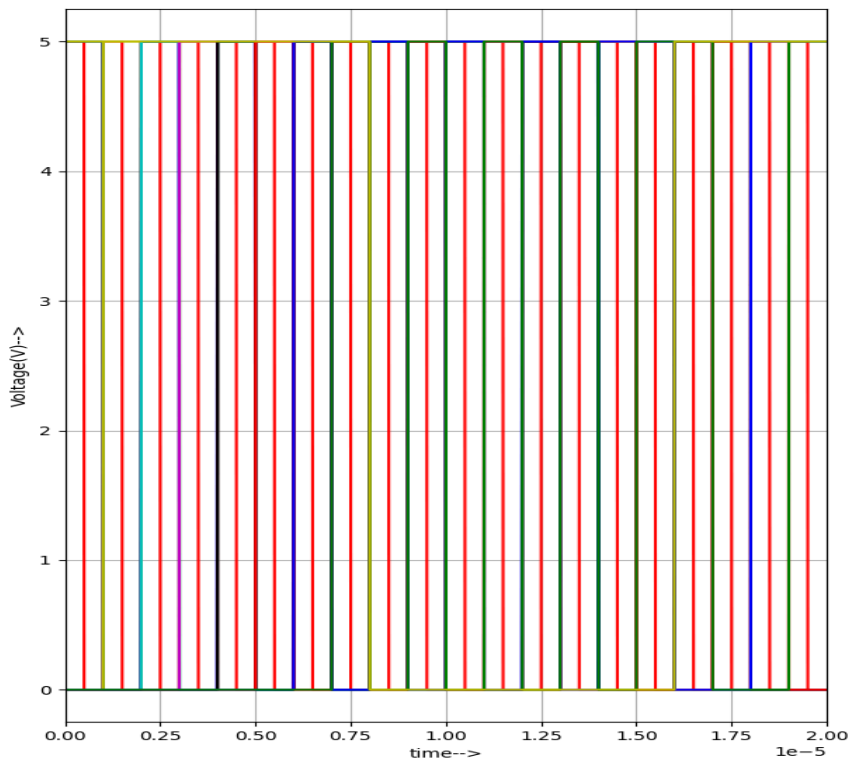
Figure 3: Full I 2 S Frame Transmission. WS = 0 (Left Channel, t = 0 to 8 \mu s) and WS = 1 (Right Channel, t = 8 \mu s to 16 \mu s) at 1 MHz SCK. Complete 16-bit stereo frame visible.
