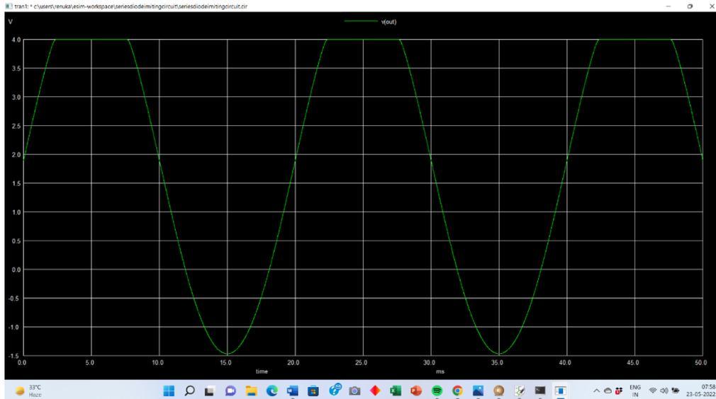
Fig. 4 Ngspice plot of output clipped voltage across the circuit
