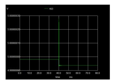
As it can be seen x and y outputs are always high, while z output goes low after 40ms mark. The exact voltage to 0 is not obtained due difficulty getting appropriate aspect ratios.
