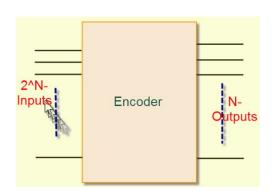
This is the basic schematic of an encoder. The input will 2<sup>N</sup> bits and the output will be N bits.
