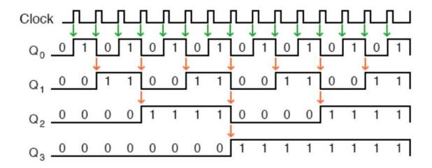
An "up" counter may be made by connecting the clock inputs of positive-edge triggered J-K flip-flops to the Q' outputs of the preceding flip-flops. The J and K inputs of all flip-flops are connected to  $V_{cc}$  or  $V_{dd}$  so as to always be "high." Counter circuits made from cascaded J-K flip-flops where each clock input receives its pulses from the output of the previous flip-flop invariably exhibit a ripple effect.
