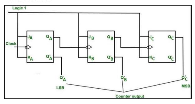
For a 3 bit asynchronous counter, 3 flip flops are required and 2<sup>3</sup>=8 states can be generated.
