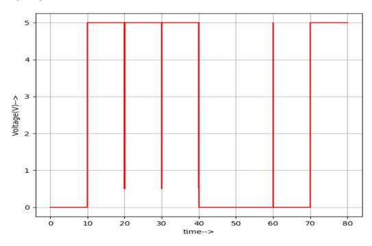
The required waveform for borrow is same as truth table.
