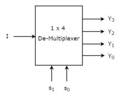
The single input 'I' will be connected to one of the four outputs, Y3 to Y0 based on the values of selection lines s1 & s0. The **Truth table** of 1x4 De-Multiplexer is shown below.
