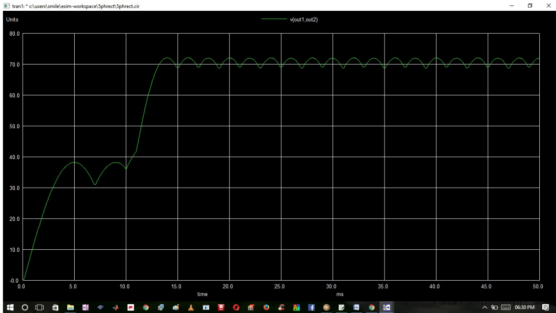
Fig 8: Ngspice plot for DC output voltage (10 pulse)
