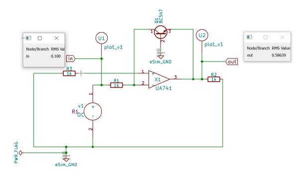
Logarithmic Amplifier Circuit Using Op-Amp with Diode in the feedback Schematic diagram:
