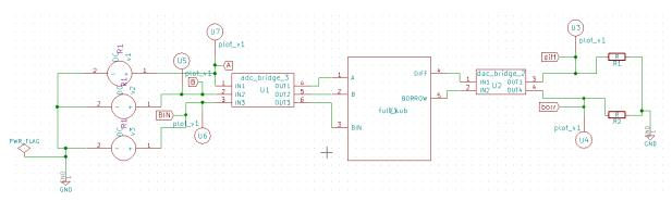
Here I used a subcircuit for subtraction. The internal structure of full subtractor is shown below.
