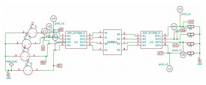
Here I used a subcircuit for two bit multiplication. The internal structure of 2 bit multiplier is shown below.
