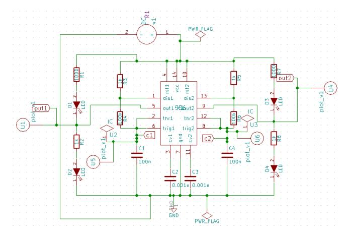
Here I used a subcircuit for IC556. The internal structure of IC556 is drawn using IC555. The diagram of subcircuit is shown below.
