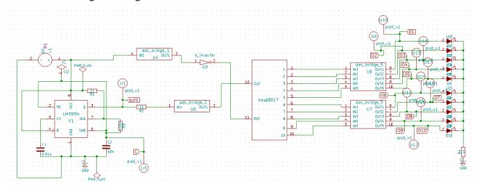
Here I used a subcircuit of LM555 and IC4017. The internal structure of this is shown below.
