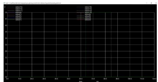
Figure 3. Alert system output. Door numbers 4,8,12,16 are open. All others are closed.
