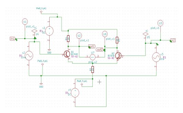
Figure 1: BJT based Differential Amplifier
